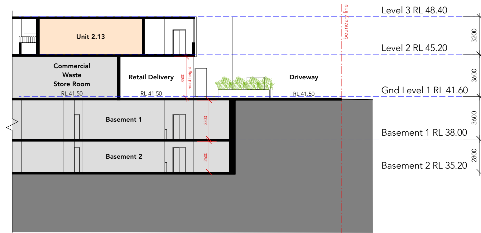
Section E-E (Retail Delivery Section)
